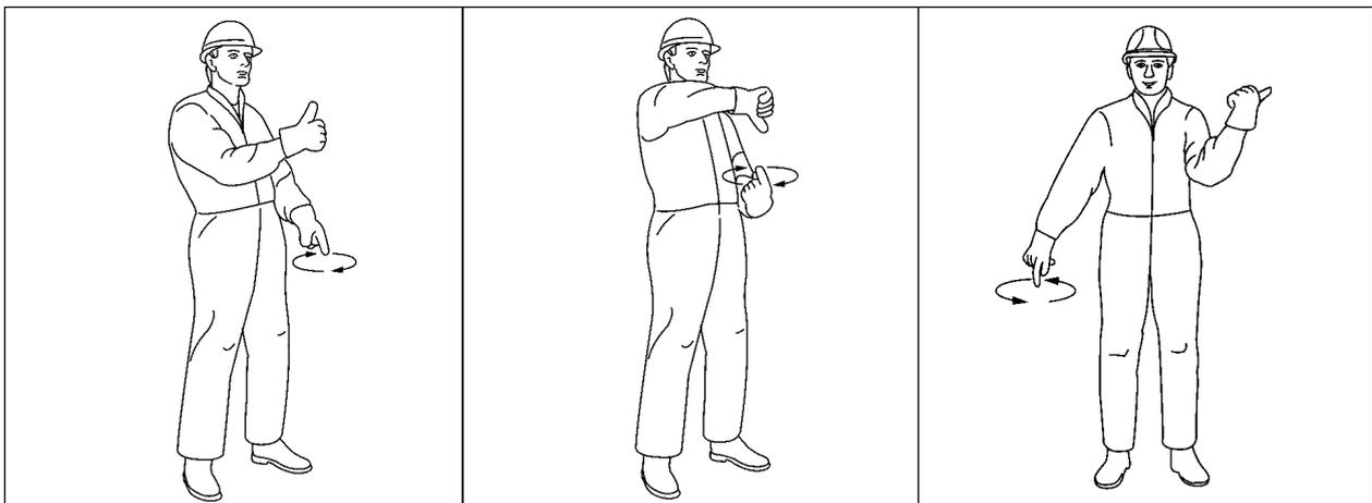
**Lift main boom and lower load**
